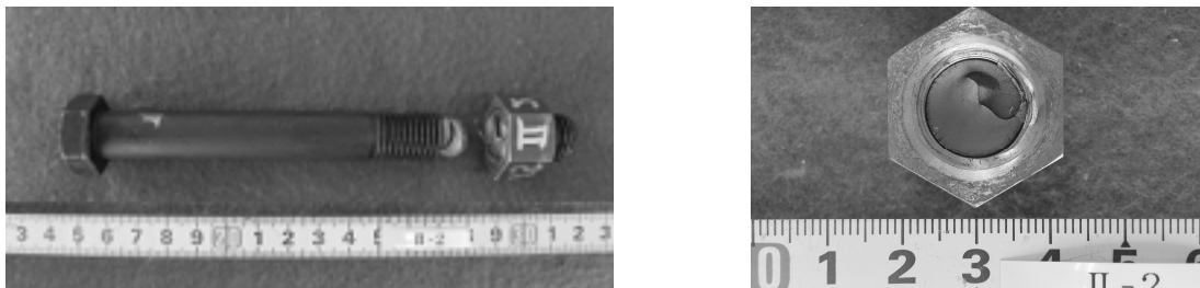
Fig. 5 Specimen ( \alpha=15\text{ }\mu\text{m} , \sigma_a=100\text{ MPa} )
