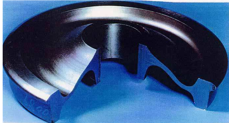
Fig. 7 New wheel, effect of ferrite volume and grain size (left), curved wheel plate (right)
