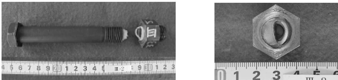
Fig. 6 Specimen ( \alpha=33\text{ }\mu\text{m} , \sigma_a=100\text{ MPa} )
