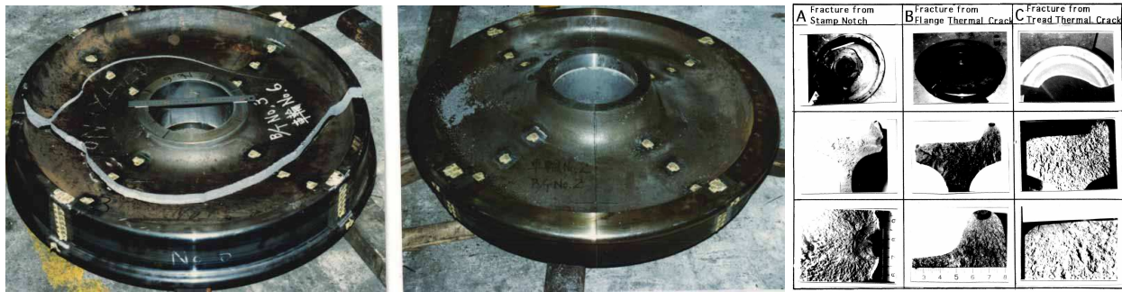
Fig. 6 Example of wheel fracture, brake testing (left), categories from stamp, flange, tread (right)
