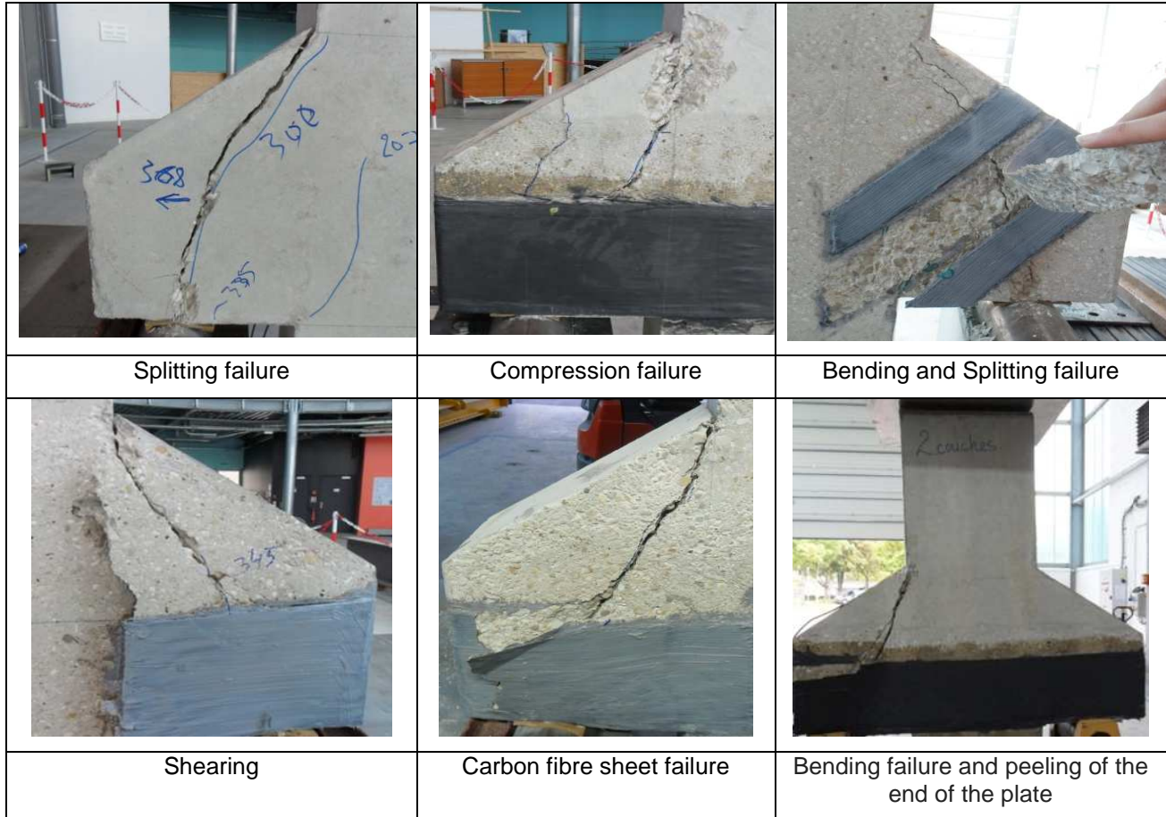
Fig. 3 Different modes of strengthening concrete short corbel failures
