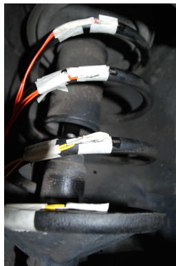
Fig. 2 1 mm size of strain gauge was used to record the strain signal
