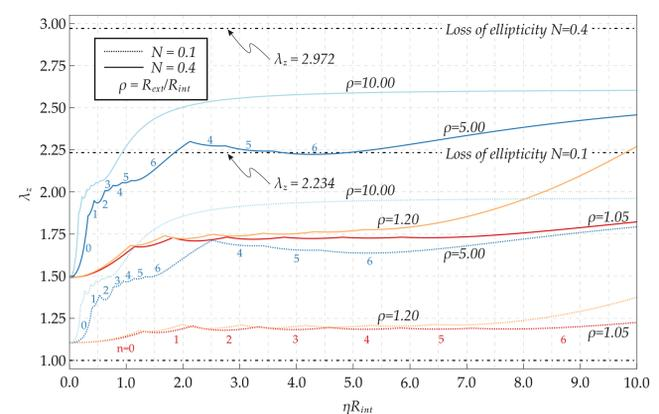
Fig. 4: Lower envelopes of the critical stretch for  $K=0.1$ , different values of the hardening exponent  $N$  and different ratios  $\rho$  as a function of  $\eta R_{int}$  ( $\eta = k\pi/L$ ,  $k=1,2,3,\dots$ ).
