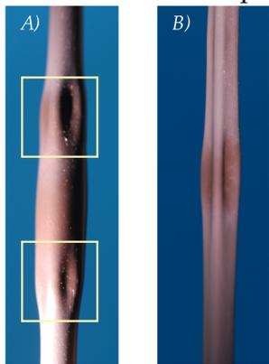
Fig. 1: Buckling under tension.
