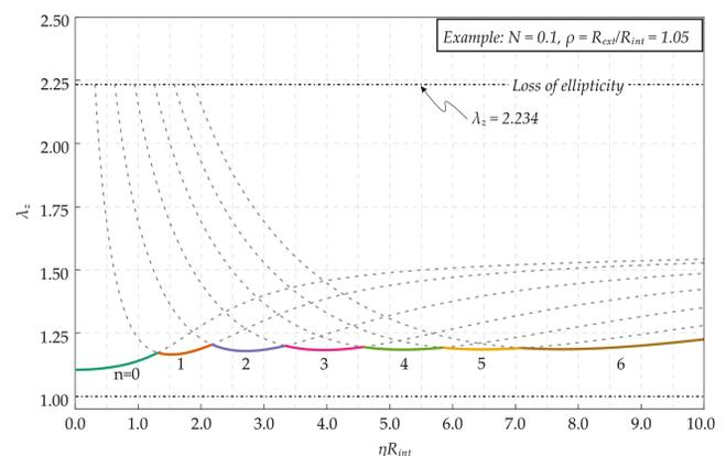
Fig. 3: Critical stretch for  $K=0.1$ ,  $N=0.1$  and  $\rho=1.05$  for different values of circumferential wave numbers  $n$  as a function of  $\eta R_{int}$  ( $\eta = k\pi/L$ ,  $k=1,2,3,\dots$ ) and lower envelope.
