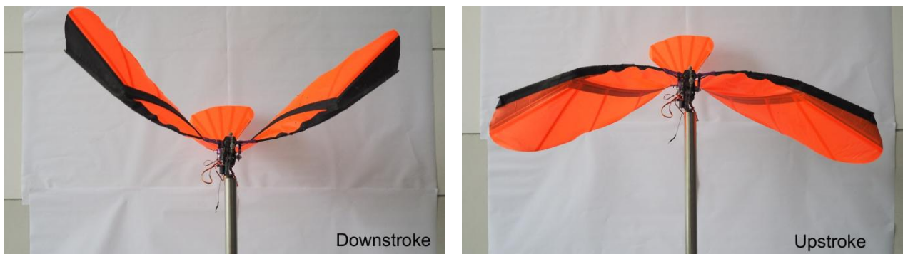
Figure 4: Side-by-side views of a single downstroke (left) and upstroke (right) of an ornithopter
