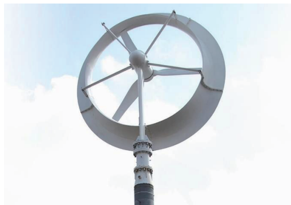
Figure 1: A wind generator with a brimmed diffuser
