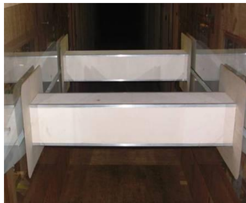
Figure 2: Two square cylinder models for spring-supported test mounted in Kyushu Institute of Technology wind tunnel
