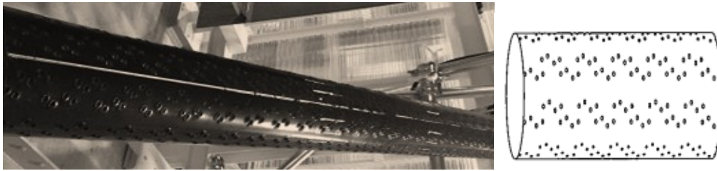
Figure 2: Indented surface cable
