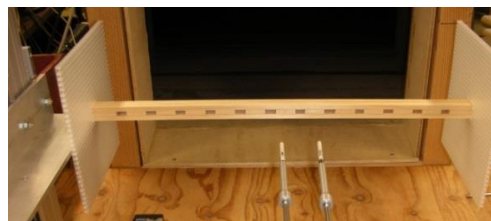
Figure 3 Model with openings and hot wires
