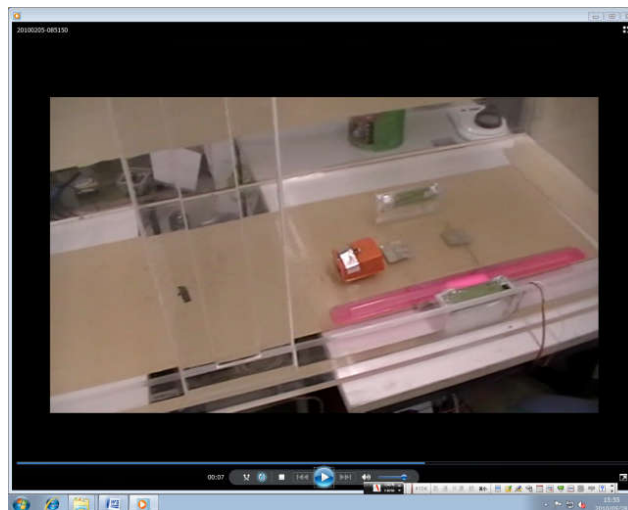
Photograph 5. Model measurement setup. The shallow water tank was constructed from acrylic plates. Paper was attached to the tank side plates to intercept extra light. The water depth was 27 mm, and the length and breadth of the tank were 1770 and 540 mm, respectively.
