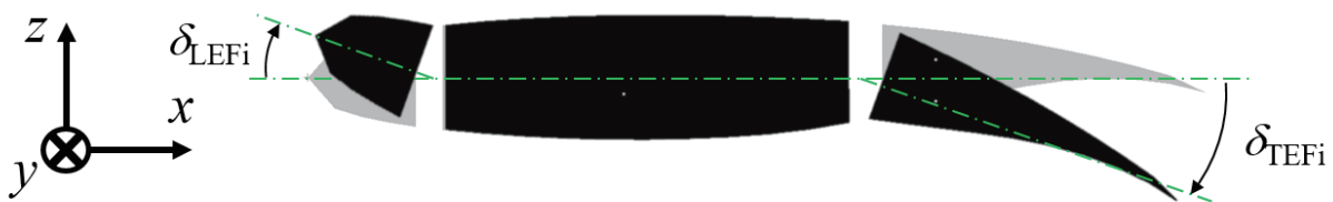
Figure 4: Definition of flap angle sign ( i=1\sim 4 ).
