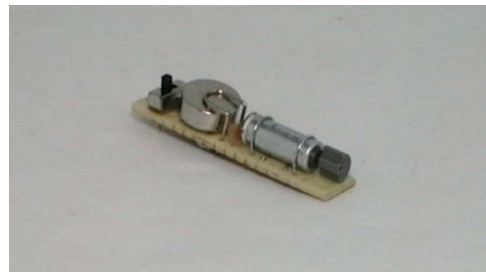
Photograph 2. Circuit of micro forced oscillator, including micro vibration motor, battery, and switch.
