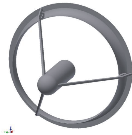
Figure 3: A brimmed diffuser shroud fixed by 3 supports
