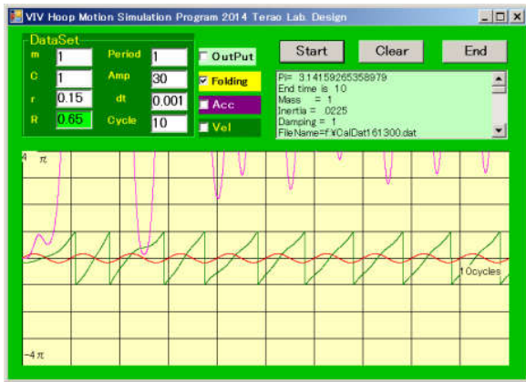
Figure 7. Sample of a diverging motion appeared in the hoop weight roll angle. The roll angle is shown from -\pi to \pi .
