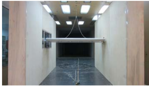
Figure 1: Spring-suspended sectional model between two fairing walls in TJ-2 wind tunnel
