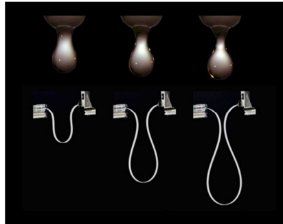
Fig. 2 The self-encapsulation or the ‘dripping’ of an elastic rod compared with the formation of a water drop
