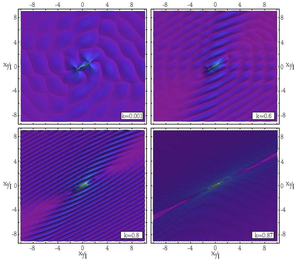
Figure 2: Real part of scattered incremental deviatoric strain at different prestress levels.
