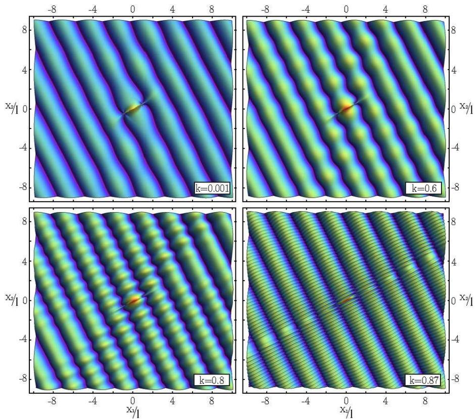
Figure 3: Real part of total incremental deviatoric strain at different prestress levels.
