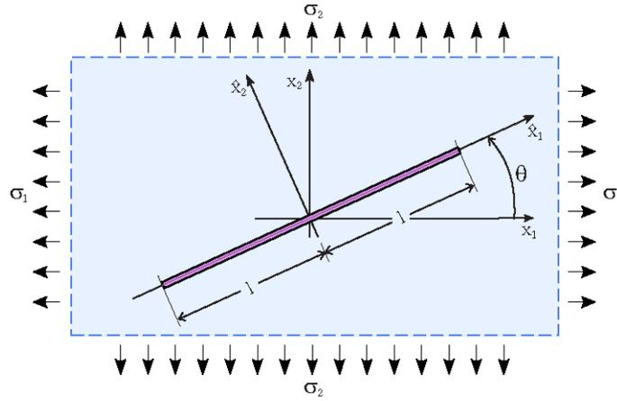
Figure 1: Shear band of finite length ( $2l$ ) and principal Cauchy stress components,  $\sigma_1$  and  $\sigma_2$ .
